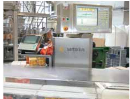
An EWK 3000 checkweigher checks product weight on the second production line
