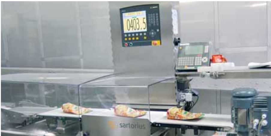
With a throughput of 100 pcs/min the SYNUS checkweigher monitors the weight of the dumpling packages
