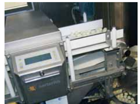
The MDP metal detector guarantees that products headed for retail are free of metal contaminants
